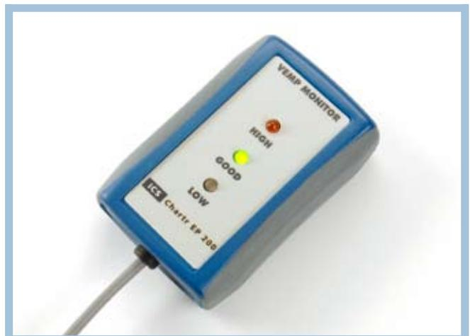
Fig. 2: VEMP Monitor with 3 light display
